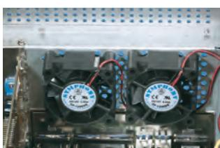
Fan 12 V DC, 60 mm, for mounting on the rear panel. Including two 4-pole connectors with terminal.
