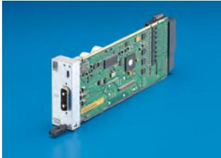
The PM is a 355 W MicroTCA PowerModule in Advanced Mezzanine Card (AMC) form factor, single/full-size compliant to MTCA.0 specification. The Power Module comprises an Enhanced Module Management Controller (EMMC) that communicates with the Carrier Manager via Intelligent Platform Management Bus (IPMB).
