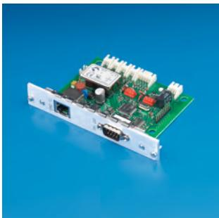
Monitoring of system voltage, PSU-status, HeiCool alarm and data transfer of the temperature- and/or fan module via the RS 232 (to PC) or RS422-interface (to CMC-TC).
